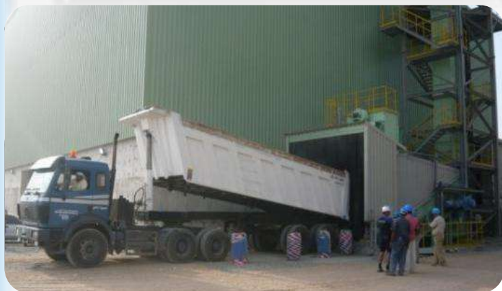
Raw material discharge via SAMSON feeder
