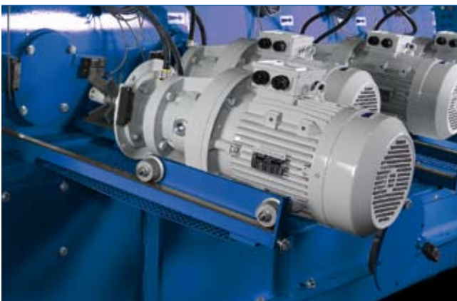
Option: agitator quick change system
